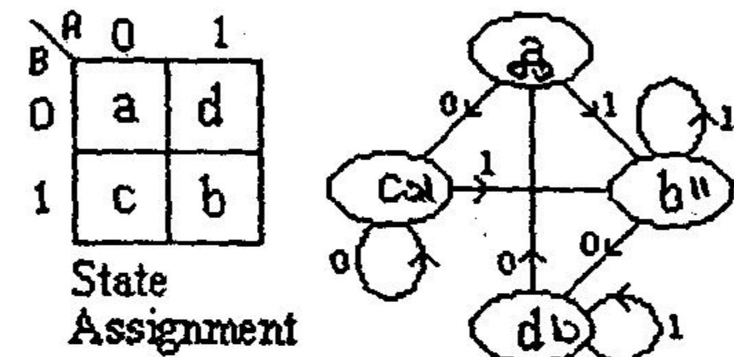
2. a. Make the state assignment in such a way as to avoid output glitches.
