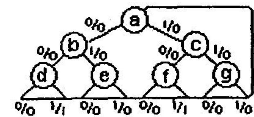
3. To what degree does the state assignment shown satisfy the 4 rules for the state transition diagram shown? (15 pts.)
