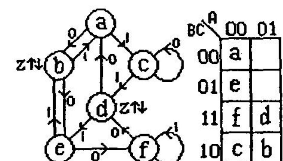
4. Realize the 4 state machine shown by the One-Hot method, using D-Flip Flops. You are free to use gates or multiplexers.
