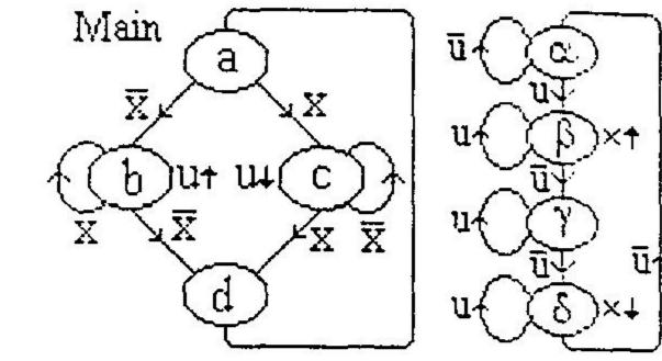
2. The figure shows a simple Asynchronous State machine, a State Transition Diagram, and two maps (M1 and M2).
