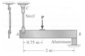
The rigid bar *AB* shown is supported by a steel rod *AC* having a diameter of 20 mm and an aluminum block having a cross- sectional area of 1800 mm<sup>2</sup>. Pins at A and C are 18-mm diameter pins. If the failure stress for the steel and aluminum is  $\sigma_{st(fail)} = 680$  MPa and  $\sigma_{AL(fail)} = 70$  MPa,
