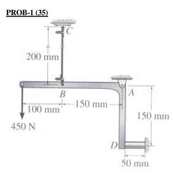
The rigid link is supported by a pin at *A*, a steel wire *BC* having an un-stretched length of 200 mm and cross-sectional area of 22.5 mm<sup>2</sup>, and a short aluminum block having an unloaded length of 50 m m and cross-sectional area of 40 mm<sup>2</sup>. If the link is subjected to the vertical load shown, determine the rotation of the link about the pin *A*. Report the answer in radians. Given that  $E_{st} = 200$  GPa and  $E_{al} = 70$  GPa.
