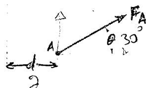
\* Max moment occurs when the force is  $\perp$  to the line between A & the point of application of the force.
