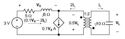
so that  $V_x = (0.1V_x - 2I_L)(5 + j5)$  and  $I_L = V_L/(-j10) = j0.1V_L$ . Substituting for  $I_L$ ,  $V_x = (0.1V_x - 2I_L)(5 + j5)$  $j(0.2V_L)(5 + j5) = 0.5V_X + j(0.5V_X - j(1 + j)V_L$ , or,  $0.5(1 - j)V_X = (1 - j)V_L$ , which gives,  $V_X = 2V_L$ . From KVL on the primary side,  $0.5V_L + 3 - V_X = 0$ ; substituting for  $V_X$ ,  $1.5V_L = 3$  and  $V_L = 2$ V.
