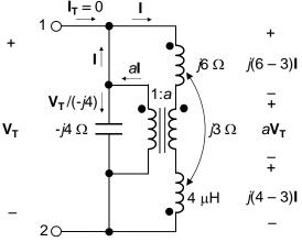
*Method 2*: The circuit can be redrawn as shown, where the two coupled coils in series have been replaced by the equivalent inductance (j6 + j4 - j6) =  $j4 \Omega$ . This
