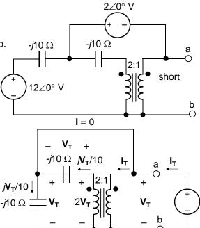
*Method 2*: Under open circuit conditions, the currents and voltages will be as shown. The voltages across the two capacitors are of equal magnitude but opposite polarity. It follows that  $2V_{Th} = 12$  V, and  $V_{Th} = 6$  V.
