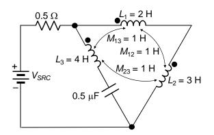
8. Given  $v_{SRC} = 6\cos\omega t$ , where  $\omega$  is unknown and k = 0.97. Determine X so that no power is dissipated in the circuit.
