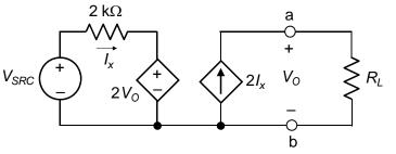
**Solution:** When terminals ab are open circuited,  $I_X = 0$ . To make  $I_X = 0$ ,  $2V_O = V_{SRC}$ , so that
