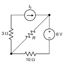
**Solution:** Since the 6 V source does not absorb or deliver any power, it follows that the current through the 6 V source and the 10  $\Omega$  resistor is zero, which means that the voltage across *R* is 6 V, and the current through *R* and the 3  $\Omega$  resistor is *I*<sub>0</sub>. It follows that the power dissipated in the resistors is  $6I_0 + 3I_0^2$ , which is also the power delivered by the source.
