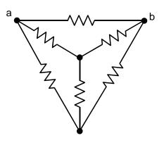
**Solution:** If the  $\Delta$  is transformed to Y, each of the resistances in Y is  $R \Omega$ , and the two Y connections are in parallel. For each Y, the resistance between nodes a and b is  $2R \Omega$ , and these in parallel give  $R \Omega$ .
