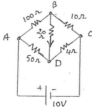
6. In problem 5, find the current flowing through the 20 Ω resistance between terminals B-D
