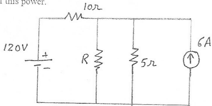
8. Find the Thevenin voltage  $V_{TH}$  shown in the circuit below
