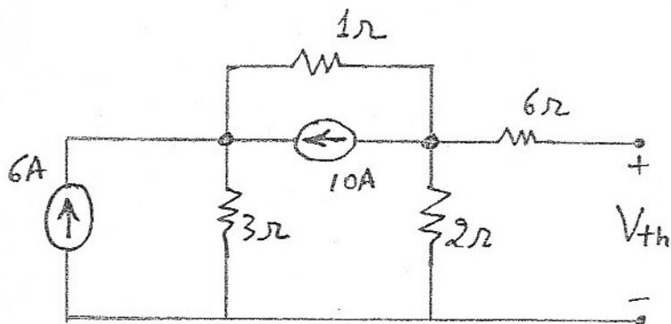
9. A network excited only by current sources is shown below. Determine the voltage at Node 1.
