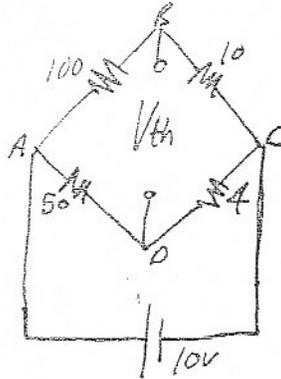
\* LET US NOW FIND THE OPEN-CIRCUIT VOLTAGE ( $V_{th}$ ). REMEMBERING THAT ABC (AS WELL AS ADC) IS A POTENTIAL DIVIDER ON WHICH A 10V DROP TAKES PLACE, WE GET:
