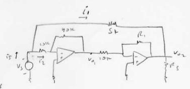
Ra does not effect The cultat supplied by source hence only constrained by power limitations & op-Amp.
