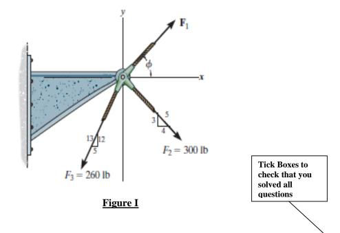
Referring to Figure I, if the magnitude of the resultant force acting on the bracket is 400 lb directed along the positive x axis, determine the magnitude of  $\mathbf{F_1}$  and its direction  $\phi$ . (15 points)
