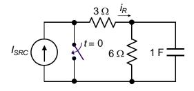
**Solution:** After the switch has been open for a long time,  $V_c = 6I_{SRC}$ . After the switch is
