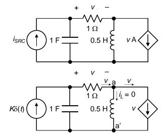
v(0) = K/1 V across the capacitor. It follows that for  $t \ge 0^+$ ,  $v(t) = Ke^{-t}$  V.
