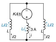
is Li + (L/2)i, where L/2 is the total inductance of the two branches in parallel and *i* is the total current in the two branches. The flux linkage in each of the two parallel branches is Li/2 Wb-Turns directed upward, the same as in the parallel combination. Since, Li = 3L, Li/2 = 1.5 L directed upward, as determined in Method 2.
