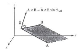
•  $\hat{n}$  direction: when the fingers of the right hand rotate from **A** to **B**; the thumb indicates **A**×**B**.
