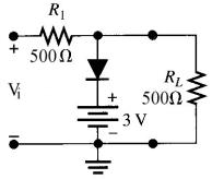
3. Find the peak inverse voltage (PIV) of the diode (in V).
