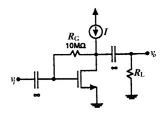
11. Find the value of the MOSFET transconductance  $g_m$  (in mA/V) if the current source carries I = 1 mA.
