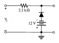
5. Find the peak inverse voltage (PIV) of the diode (in V).
