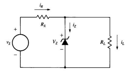
13. What is the maximum value of  $R_X$  (in  $\Omega$ ) for which the Zener diode remains in the breakdown region?
