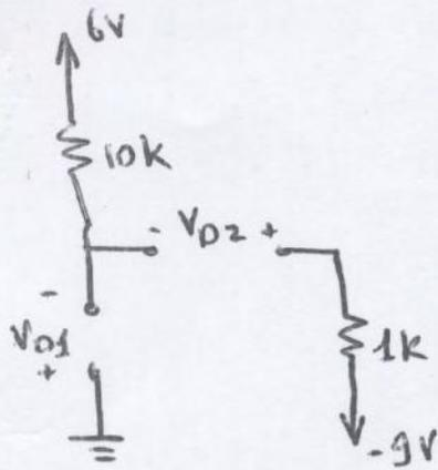
$$\text{KVL} \Rightarrow 6 = 10\text{k} \times 0 - V_{D1} \Rightarrow V_{D1} = -6\text{V} < 0 \Rightarrow D_1 \text{ off}$$
