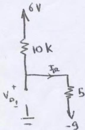
$$I_{D2} = \frac{6 - (-9)}{(10 + 5) \text{ k}} = \frac{15}{15 \text{ k}} = 1 \text{ mA} > 0 \Rightarrow \text{correct assumption}$$
