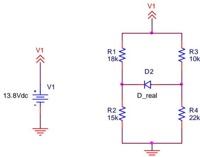
To simulate the circuit now with a real diode, right-click on the diode symbol, then click on Edit Pspice Model. Replace the `.model` line in the Model Editor with the following line:
