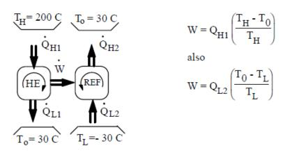
$$\frac{Q_{H1}}{Q_{L2}} = \left(\frac{T_o - T_L}{T_L}\right) \left(\frac{T_H}{T_H - T_o}\right) = \left(\frac{60}{243.2}\right) \left(\frac{473.2}{170}\right) = \mathbf{0.687}$$
