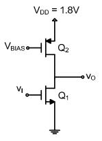
The technology parameters are:  $k'_n = 300 \ \mu A/V^2$ ,  $V_{tn} = 0.45 \ V$ ,  $V_{An} = 5 \ V$ ,  $k'_p = 100 \ \mu A/V^2$ ,  $V_{tp} = -0.5 \ V$ , and  $|V_{Ap}| = 4 \ V$ .
