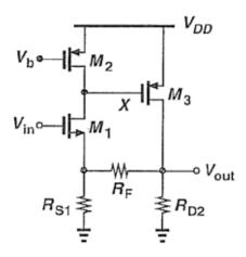
(a) Determine the input bias voltage required to establish the above currents.
