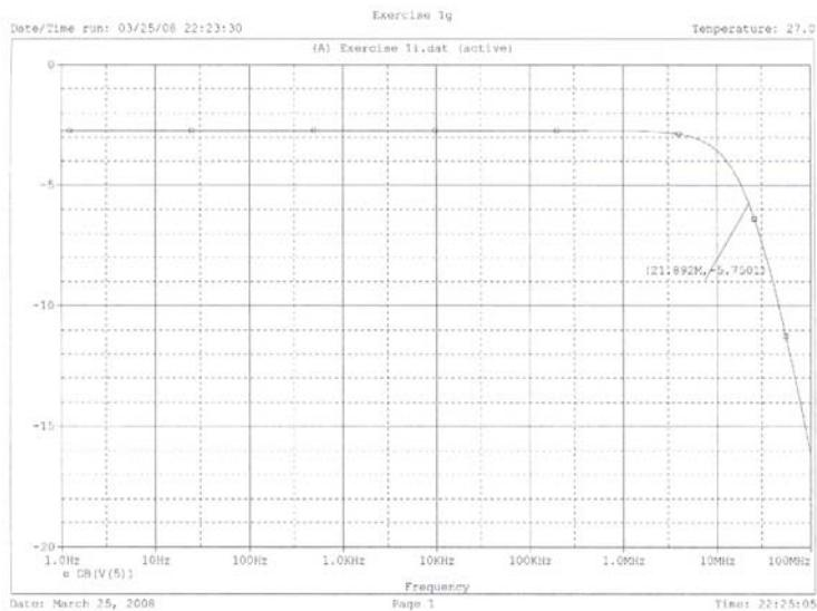
The 3db frequency from the bode plot is 21.892 MHz which is really close to the one we calculated which is 21.84 MHz.
