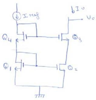
$$\begin{aligned}I_{REF} &= 10 \mu A \\V_o &= 2,5 V \\K_n^2 \frac{W}{L} &= 1 \text{ mA/V}^2 \\V_t &= 0,5 V \\V_A &= 10 V\end{aligned}$$
