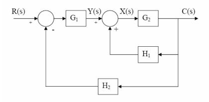
Write an M file that computes the transfer function C(s)/R(s) of the system above given that:  $G_1 = \frac{s^2 + 3s + 5}{s^3 + 2s + 1}$ ;  $G_2 = 4$ ;  $H_1 = \frac{1}{s + 4}$ ; and
