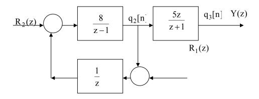
$\begin{aligned} q_1[n+1] &= q_2[n] + r_2[n] \\ q_2[n+1] &= 8q_1[n] + q_2[n] + 8r_2[n] \\ q_3[n+1] &= 40q_1[n] + 5q_2[n] - q_3[n] + 40r_2[n] \end{aligned}$
