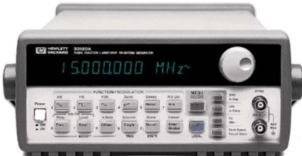
Figure D-1: HP Agilent 33120A Function generator
