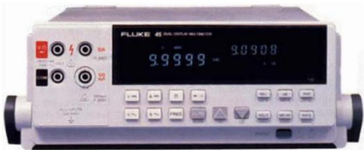
Figure C-1 The Fluke 45 DMM
