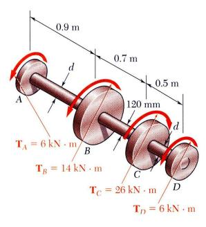
Shaft *BC* is hollow with inner and outer diameters of 90 mm and 120 mm, respectively. Shafts *AB* and *CD* are solid of diameter *d*. For the loading shown, determine (*a*) the minimum and maximum shearing stress in shaft *BC*, (*b*) the required diameter *d* of shafts *AB* and *CD* if the allowable shearing stress in these shafts is 65 MPa.
