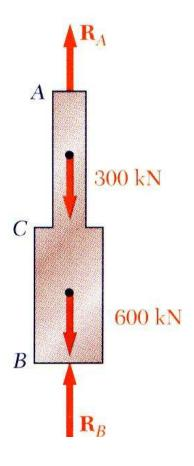
Require that the displacements due to the loads and due to the redundant reaction be compatible,
