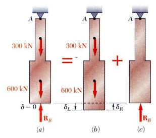
Determine the reactions at A and B for the steel bar and loading shown, assuming a close fit at both supports before the loads are applied.
