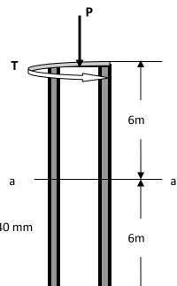
c-At section a-a, the axial compressive load is the sum of the external load P and the weight of upper part of the shaft form the top to the middle section
