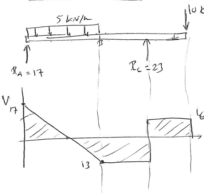
$$V_{max} = 17 \text{ kN}$$
