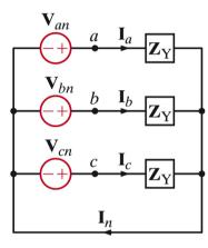
Positive sequence, balanced Y-Y three-phase circuit. Source  $V_{\phi}=120$  Vrms.  $\hat{Z}_{line}=1+j1$   $\Omega$ .  $\hat{Z}_{Y}=20+j10$   $\Omega$ .
