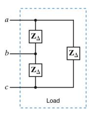
A three-phase balanced wye-delta system has a line voltage magnitude of 208 Vrms. The line impedance is negligible. The total real power absorbed by the load is 1200 W and the power factor angle of the load is 20°. Determine the magnitude of the line current and the value of the load impedance per phase in the delta.
