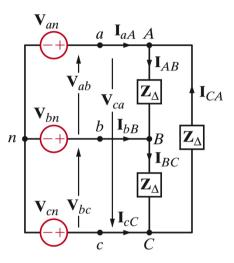
A delta-connected load consists of 10  $\Omega$  resistance in series with 20 mH inductance. The source is Y-connected, abc sequence, 60 Hz,  $\tilde{V}_{an}=120 \angle 30^\circ$  Vrms. Determine the line currents and the phase currents in the  $\Delta$ -connected load.
