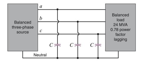
Example: in the previous diagram, f=60 Hz,  $V_L=34.5$  kVrms, required PF = 0.9 lagging. Find C.
