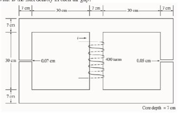
Sclutton. This core can be divided up into five regions. Let  $\mathcal{R}_1$  be the reluctance of the left-hand portion of the core,  $\mathcal{R}_3$  be the reluctance of the left-hand air gap,  $\mathcal{R}_3$  be the reluctance of the right-hand portion of the core,  $\mathcal{R}_4$  be the reluctance of the right-hand air gap, and  $\mathcal{R}_5$  be the reluctance of the center leg of the core. Then the total reluctance of the core is
