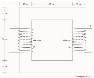
Solution The two coils on this core are would so that their magnetomotive forces are additive, so the total magnetomotive force on this core is
