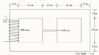
Solution. This core can be divided up into four regions. Let  $\mathcal{R}_1$  be the reluctance of the left-hand portion of the core,  $\mathcal{R}_2$  be the reluctance of the center leg of the core,  $\mathcal{R}_3$  be the reluctance of the center air gap, and  $\mathcal{R}_4$  be the reluctance of the right-hand portion of the core. Then the total reluctance of the core is
