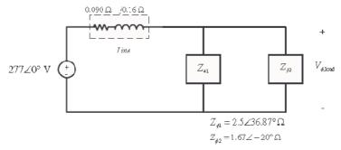
(a) The phase voltage of the equivalent Y-loads can be found by nodal analysis.
