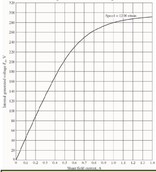
Note: An electronic version of this magnetization curve can be found in file  $p91\_mag.dat$ , which can be used with MATLAB programs. Column 1 contains field current in amps, and column 2 contains the internal generated voltage  $E_A$  in volts.
