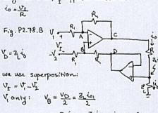
$$\frac{V_{i} - \frac{3L\dot{c}_{0}}{2}}{R_{i}} = \frac{\frac{3L\dot{c}_{0}}{2} - \dot{c}_{0}(2L + R)}{R_{i}}$$
