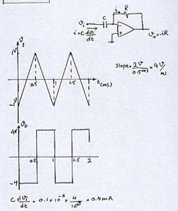
Thus the peak value of the output squere wave is 0.4mAx10<sup>k,II</sup>=4V. The frequency of the output is the same as the input (1KH2).
