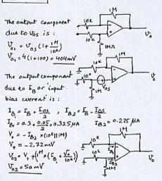
The worst case (largest) DC offset voltage at the output is 404+50=454mV
