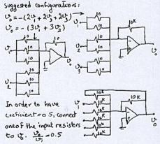
The output signal should be:  $V = -5\sin\omega t - 5$ if we assume:  $V_1 = 5\sin\omega t$   $V_2 = 2V$ In a weighted sommer configuration:  $\frac{Re}{R_1} = +1$   $\frac{Re}{R_2} = 2.5$   $R_2 = 10KR \Rightarrow R_1 = 25K = R_1$   $V = \frac{R_2 = 25K}{V_2}$   $V = \frac{R_2 = 25K}{V_2}$
