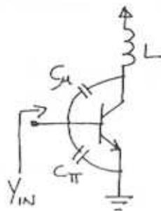
for  $\omega C_{\mu} \ll \frac{1}{\omega L}$
