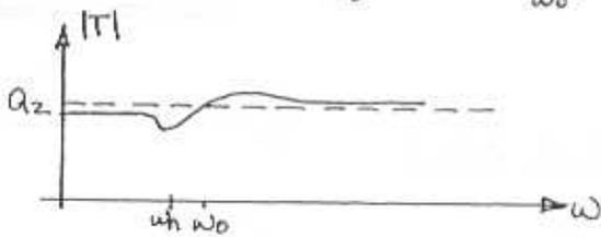
If zero frequency > pole frequency then  $\omega_n > \omega_0$
