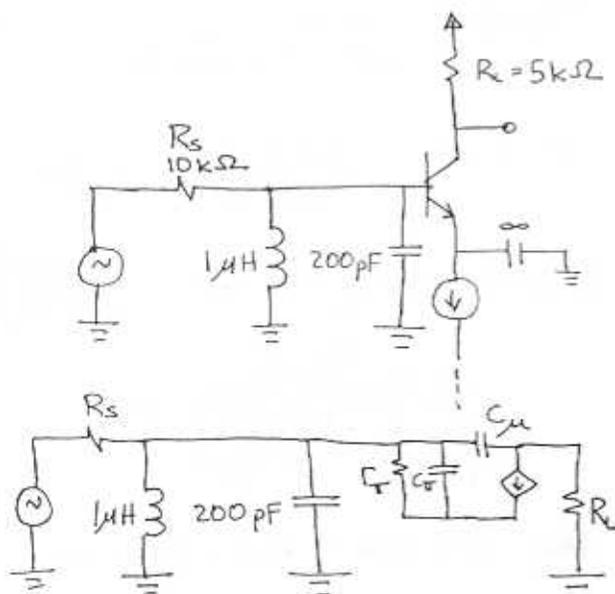
$$r_e = 25 \Omega, C_{\mu} = 1 \text{ pF}, C_{\pi} = 10 \text{ pF}, \beta = 200$$
