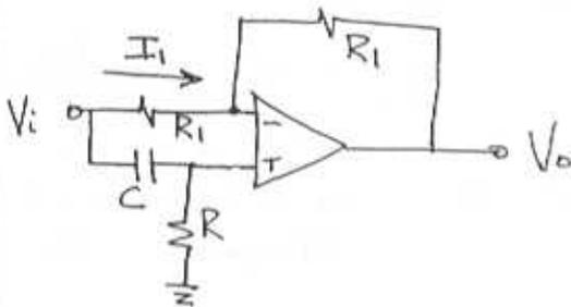
$$V_+ = \frac{R}{R + 1/sC} V_i = \frac{s}{s + \omega_0} V_i$$
