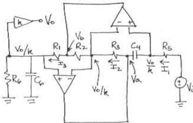
Because of the virtual short at opamp input terminals, the voltages are:  $V_o/k$
