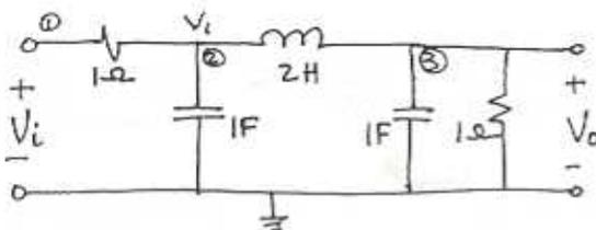
The easiest way to solve the circuit is to use nodal analysis at nodes ①, ②, ③
