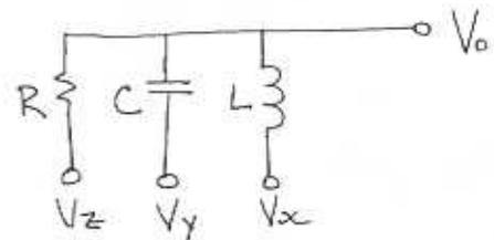
$$\left. \frac{V_o}{V_z} \right|_{V_y = V_x = 0} = T_{BP}(s)$$
