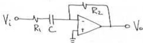
$$R_i(\infty) = R_1 = \underline{100 \text{ k}\Omega}$$
