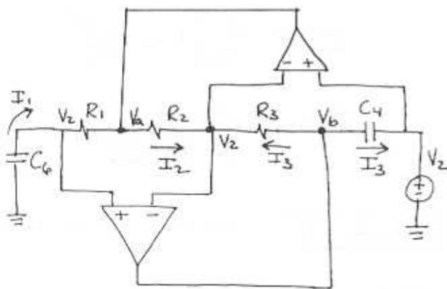
Because of virtual short at opamp input terminals all nodes are at  $V_2$ !
