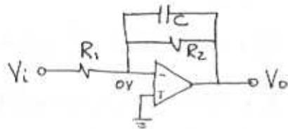
$$R_{in} = R_1 = \underline{10 \text{ k}\Omega}$$
