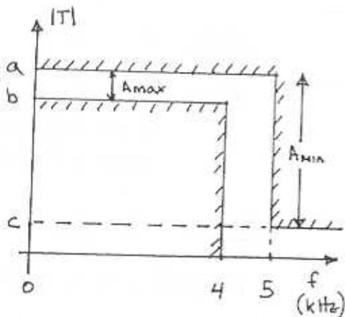
Note  $|T|$  is shown in a linear scale but  $A_{max}$  and  $A_{min}$  are in dB
