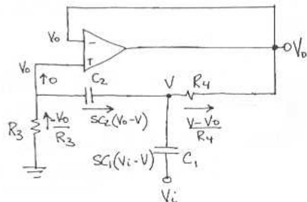
∵ No current can't flow into +ve terminal
