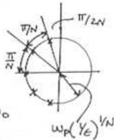
$$P_1 = \omega_0 \angle \left( \frac{\pi}{2} + \frac{\pi}{2N} \right) = \omega_0 \angle \left( \frac{6\pi}{10} \right)$$
