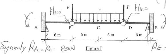
For the beam shown in Figure I, the own weight is neglected.
