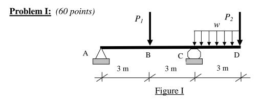
Referring to <u>Figure I</u>, let *EI*=50,000 kN.m<sup>2</sup> throughout the beam. Neglect the own weight of the beam.
