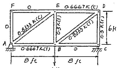
[b] Determine the vertical displacement of joint E. For each member  $A = 1.5 \text{ in}^2$ ,  $E = 29(10^3) \text{ ksi}$ . Use the method of virtual work.
