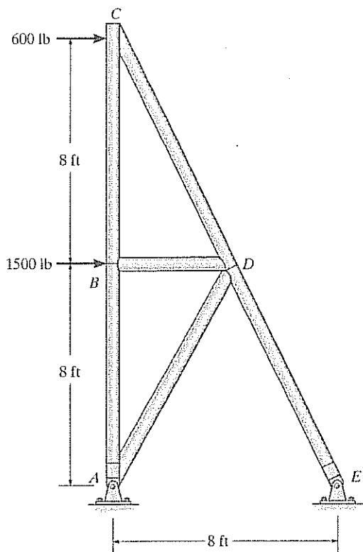
[c] Remove the loads on the truss in Prob. 9-42 and determine the horizontal displacement of point C if member CD is fabricated 0.5 in. too short.
