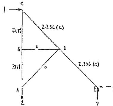
[b] Remove the loads on the truss in Prob. 9-42 and determine the horizontal displacement of point C if members AB and BC experience a temperature increase of  $\Delta T = 200^{\circ}\text{F}$ . Take  $A = 2 \text{ in}^2$  and  $E = 29(10^3) \text{ ksi}$ . Also,  $\alpha = 10^{-6}/^{\circ}\text{F}$ .
