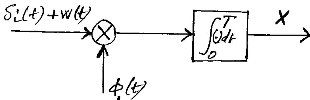
$$X = \begin{cases} 2A\sqrt{T} + W_1, & \text{if } S_1(t) \text{ is sent} \\ A\sqrt{T} + W_1, & \text{if } S_2(t) \text{ is sent} \\ -A\sqrt{T} + W_1, & \text{if } S_3(t) \text{ is sent} \\ -2A\sqrt{T} + W_1, & \text{if } S_4(t) \text{ is sent.} \end{cases}$$
