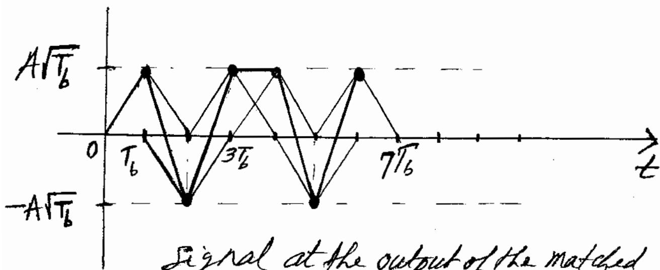
Signal at the output of the matched filter before sampling.
