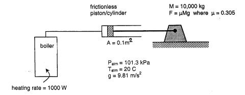
a) the piston will begin moving when the pressure inside the sufficient to overcome the fuetion force and atmospheric pressure.
