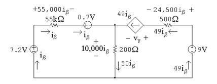
**[a]** To find  $i_{\beta}$ , write a KVL equation around the left-hand loop, summing voltages in a clockwise direction starting below the 7.2V source:
