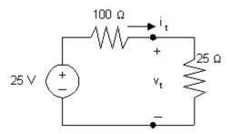
To find the power delivered to the  $25 \Omega$  resistor we must calculate the current through the  $25 \Omega$  resistor. Do this by first using KCL to recognize that the current in each of the components is  $i_t$ , flowing in a clockwise direction. Write a KVL equation in the clockwise direction, starting below the voltage source, and using Ohm's law to express the voltage drop across the resistors in the direction of the current  $i_t$  flowing through the resistors:
