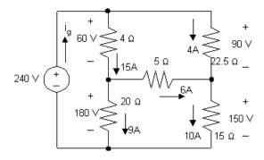
Calculate the power dissipated by the resistors using the equation  $p_R = Ri_R^2$ :  $p_{4\Omega} = (4)(15)^2 = 900 \text{ W}$   $p_{20\Omega} = (20)(9)^2 = 1620 \text{ W}$   $p_{5\Omega} = (5)(6)^2 = 180 \text{ W}$   $p_{22.5\Omega} = (22.5)(4)^2 = 360 \text{ W}$  $p_{15\Omega} = (15)(10)^2 = 1500 \text{ W}$
