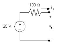
**[b]** Draw the circuit model from part (a) and attach a  $25 \Omega$  resistor:
