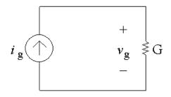
[a] Note from the circuit that the current throught the conductance G is  $i_g$ , flowing from top to bottom (from KCL), and the voltage drop across the current source is  $v_q$ , positive at the top (from KVL). From a version of Ohm's law,
