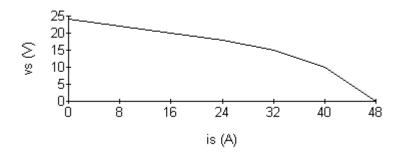
**[b]** Since the plot is linear for  $0 \le i_s \le 24$  A and since  $R = \Delta v / \Delta i$ , we can calculate R from the plotted values as follows:
