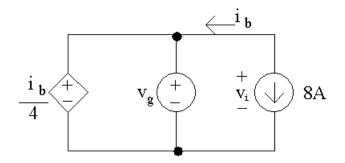
[a] To find  $v_g$  write a KVL equation clockwise around the left loop, starting below the dependent source:
