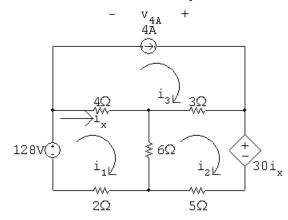
There is a current source on the perimeter of the  $i_3$  mesh, so  $i_3 = 4$  A. The other two mesh current equations are
