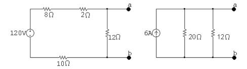
Finally, combine the 20  $\Omega$  and 12  $\Omega$  parallel resistors to give  $R_{\rm N} = 20 || 12 = 7.5 \Omega$ . Thus, the Norton equivalent circuit is the parallel combination of a 6 A source and a 7.5  $\Omega$  resistor.
