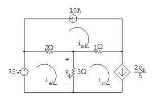
There are current sources on the perimeters of both the  $i_{\rm b}$  mesh and the  $i_{\rm c}$  mesh, so we know that
