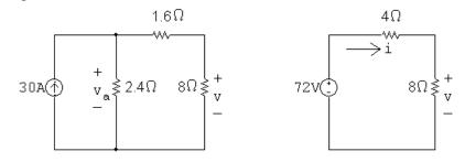
Use voltage division in the circuit on the right to calculate v as follows:
