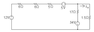
Now combine the 12 V and 5 V sources into a single voltage source and the  $6\Omega$ ,  $6\Omega$  and  $5\Omega$  resistors into a single resistor to get
