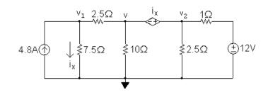
Note that the dependent voltage source and the node voltages v and  $v_2$  form a supernode. The  $v_1$  node voltage equation is
