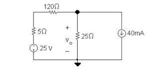
Note that we have chosen the lower node as the reference node, and that the voltage at the upper node with respect to the reference node is  $v_o$ . Write a KCL equation (node voltage equation)by summing the currents leaving the upper node:
