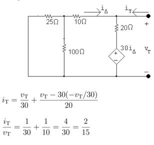
$$R_{\rm Th} = \frac{v_{\rm T}}{i_{\rm T}} = \frac{15}{2} = 7.5\,\Omega$$
