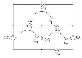
The 2 A current source is shared by the meshes  $i_{\rm a}$  and  $i_{\rm b}$ . Thus we combine these meshes to form a supermesh and write the following equation:
