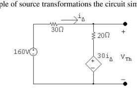
$$i_{\Delta} = \frac{160 - 30i_{\Delta}}{50}; \qquad i_{\Delta} = 2 \text{ A}$$
