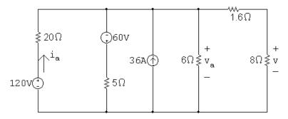
Transform the 120 V source in series with the 20  $\Omega$  resistor into a 6 A source in parallel with the 20  $\Omega$  resistor. Also transform the -60 V source in series with the 5  $\Omega$  resistor into a -12 A source in parallel with the 5  $\Omega$  resistor. The result is the following circuit:
