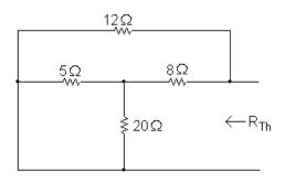
Note that the 5  $\Omega$  and 20  $\Omega$  resistors are in parallel, with an equivalent resistance of  $5||20 = 4 \Omega$ . The equivalent  $4 \Omega$  resistance is in series with the  $8 \Omega$  resistor for an equivalent resistance of  $4 + 8 = 12 \Omega$ . Finally, the  $12 \Omega$  equivalent resistance is in parallel with the  $12 \Omega$  resistor, so  $R_{\rm Th} = 12||12 = 6 \Omega$ .
