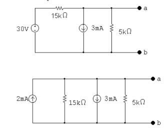
Therefore the Norton equivalent is determined by adding the current sources and combining the resistors in parallel:
