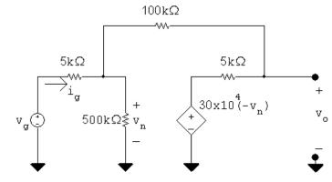
AP 5.6 [a] Replace the op amp with the more realistic model of the op amp from Fig. 5.15:
