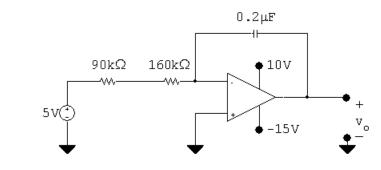
$$v_o = -\frac{1}{RC_f} \int_{32 \times 10^{-3}}^t 5\,dy + 8 = -\frac{1}{RC_f} (5y) \Big|_{32 \times 10^{-3}}^t + 8 = -\frac{1}{RC_f} 5(t - 32 \times 10^{-3}) + 8$$
