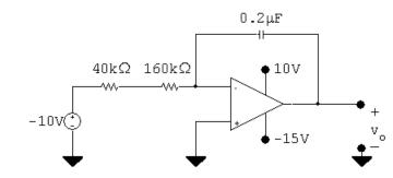
$$v_o = -\frac{1}{RC_f} \int_0^{32 \times 10^{-3}} -10 \, dt + 0 = -\frac{1}{RC_f} (-10t) \Big|_0^{32 \times 10^{-3}} = -\frac{1}{RC_f} (-320 \times 10^{-3})$$
