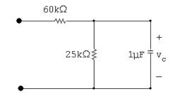
For  $0 \le t \le 100 \text{ ms}$ :  $\tau = RC = (25 \times 10^3)(1 \times 10^{-6}) = 25 \text{ ms}$  $v_c(t) = v_c(0^-)e^{t/\tau} = 80e^{-40t} \text{ V}, \qquad 0 \le t \le 10 \text{ ms}$
