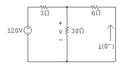
First combine the  $30 \Omega$  and  $6 \Omega$  resistors in parallel:
