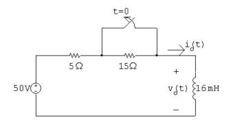
For t < 0, the  $15 \Omega$  resistor is by passed:
