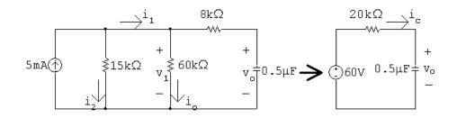
Since there is no source connected to the capacitor for t < 0
