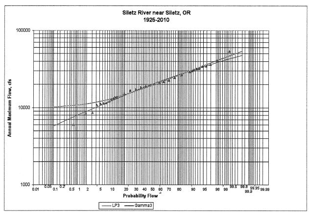
**3.10** Using graphs from Problem 3.9 and additional computations as appropriate, estimate the return period and nonexceedance probability, of a flood of magnitude 30,000 cfs for the Siletz River, 1925 - 2010.
