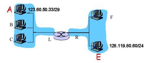
a) Write down an IP address for each interfaces at all hosts and routers in the diagram. Note that the IP addresses and network prefix for A and E are as given. Remember to consider the fact that the addresses containing all ones and all zeros for the host part of the address are reserved and cannot be assigned to interfaces.
