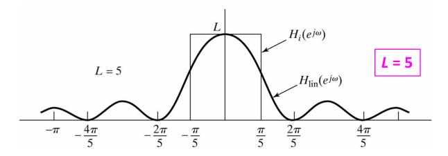
If original sampling rate greatly exceeds Nyquist rate, signal will not vary significantly between samples, and hence linear interpolation will be more accurate for oversampled signals
