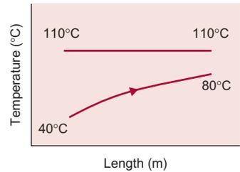
■ **Figure E4.18** Temperature plots for a parallel-flow heat exchanger.
