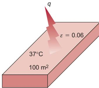
■ Figure E4.5 Heat transfer from a plate.
