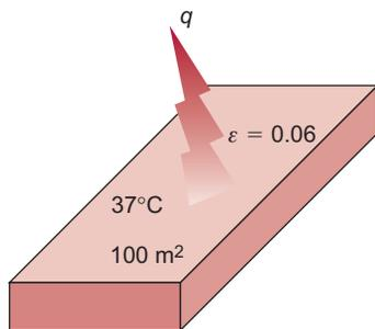
■ Figure E4.5 Heat transfer from a plate.
