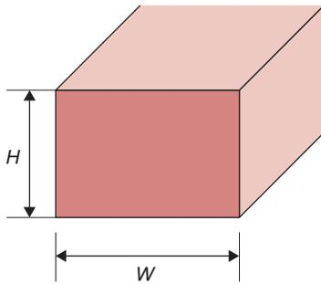
■ **Figure 4.24** Cross-section of a rectangular duct.
