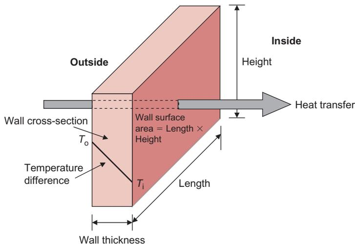
■ Figure 4.11 Conductive heat flow in a wall.
