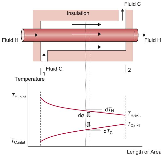
■ **Figure 4.28** A concurrent flow heat exchanger and temperature plots.
