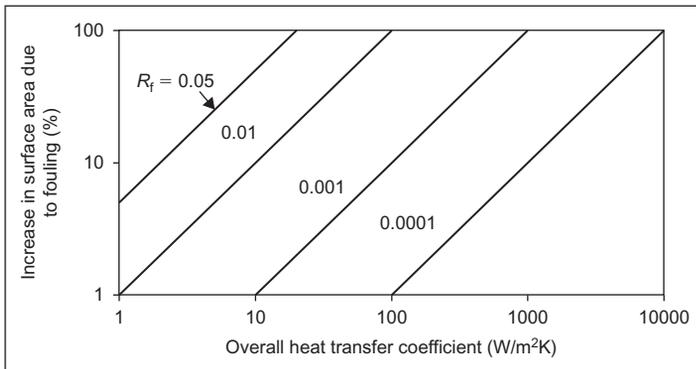
■ **Figure E4.15** Increase in surface area due to fouling.
