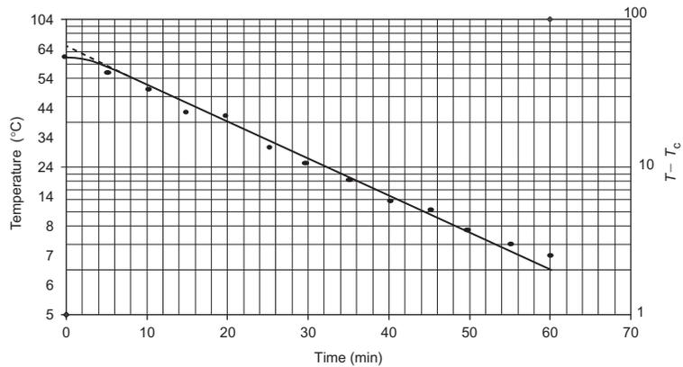
3. Determine the time for the straight line to traverse one log cycle to obtain  $f_c$ . From the plot we get  $f_c = 40$  min.
