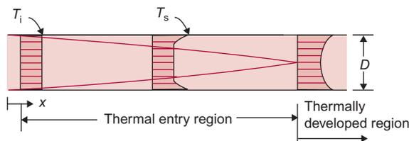
■ **Figure 4.19** Thermal entry region in fluid flowing in a pipe.
