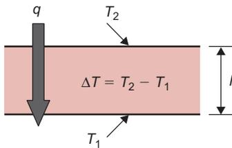
■ **Figure 4.20** Heat transfer through a fluid layer.
