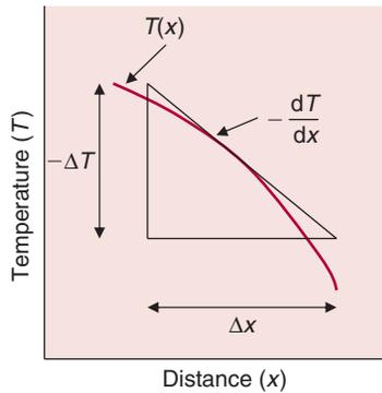
■ **Figure 4.12** Sign convention for conductive heat flow.
