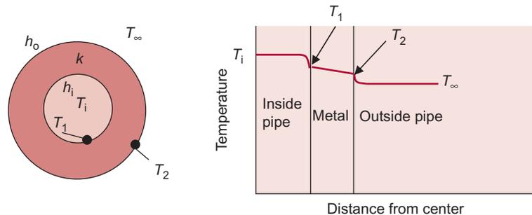
where  $k$  is the thermal conductivity of the pipe material (W/[m K]),  $r_i$  is the inside radius (m), and  $r_o$  is the outside radius (m). Resistance to heat transfer due to convection at the outside pipe surface is
