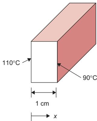
■ **Figure E4.3** Heat flow in a plate.
