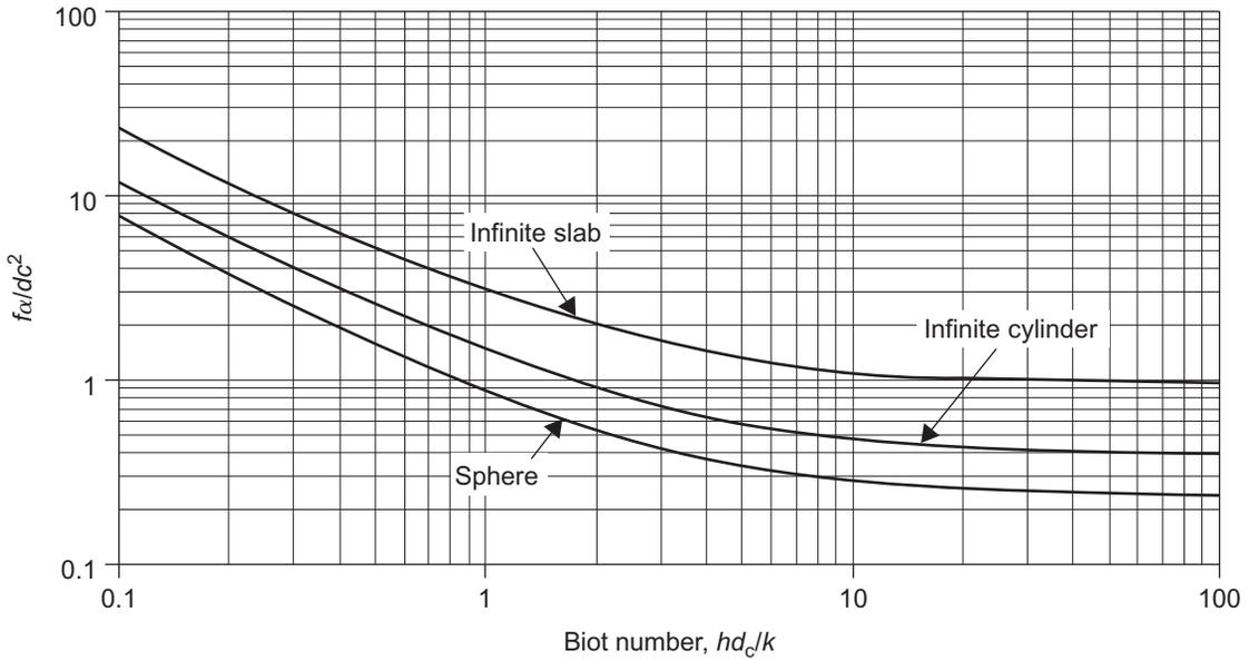
**W** **Figure 4.40** Heating rate parameter,  $f_h$ , as a function of Biot number.
