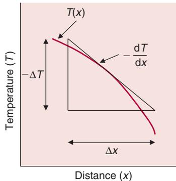
■ **Figure 4.12** Sign convention for conductive heat flow.
