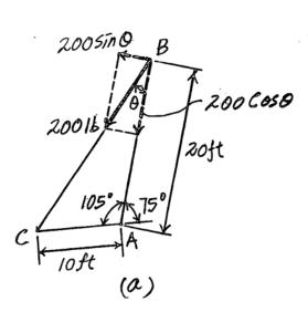
•4–25. In order to raise the lamp post from the position shown, the force **F** on the cable must create a counterclockwise moment of 1500 lb  $\cdot$  ft about point *A*. Determine the magnitude of **F** that must be applied to the cable.
