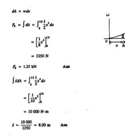
•4–153. Wet concrete exerts a pressure distribution along the wall of the form. Determine the resultant force of this distribution and specify the height h where the bracing strut should be placed so that it lies through the line of action of the resultant force. The wall has a width of 5 m.
