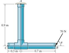
\*4–28. The 70-N force acts on the end of the pipe at *B*. Determine the angles  $\theta$  (0°  $\leq \theta \leq 180^{\circ}$ ) of the force that will produce maximum and minimum moments about point *A*. What are the magnitudes of these moments?
