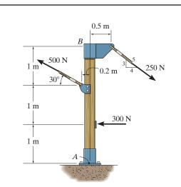
\*4–128. Replace the force system acting on the post by a resultant force, and specify where its line of action intersects the post AB measured from point B.
