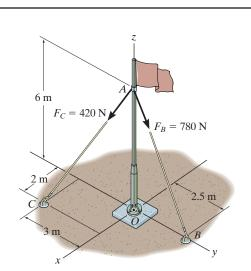
**Position Vector and Force Vectors:** The position vector  $\mathbf{r}_{OA}$  and force vectors  $\mathbf{F}_B$  and  $\mathbf{F}_C$ , Fig. *a*, must be determined first.
