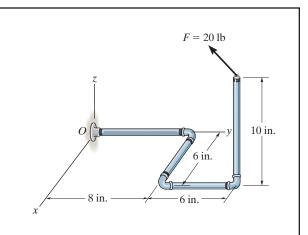
•4–165. Determine the moment of the force **F** about point *O*. The force has coordinate direction angles of  $\alpha = 60^{\circ}$ ,  $\beta = 120^{\circ}$ ,  $\gamma = 45^{\circ}$ . Express the result as a Cartesian vector.
