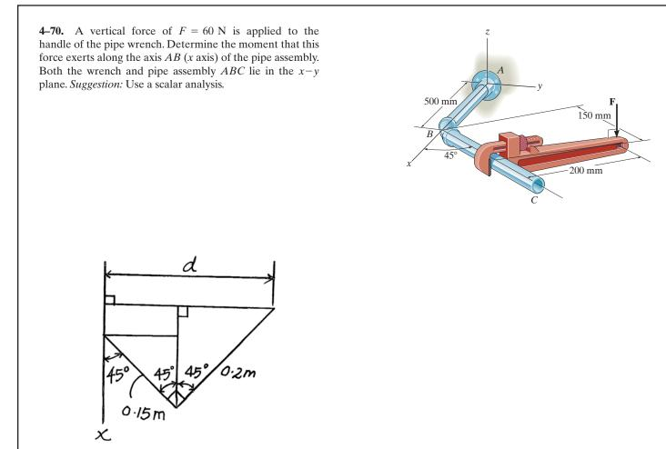
Scalar Analysis: From the geometry, the perpendicular distance from x axis to force F is  $d = 0.15 \sin 45^\circ + 0.2 \sin 45^\circ = 0.2475$  m.
