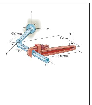
Scalar Analysis : From the geometry, the perpendicular distance from x axis to F is  $d = 0.15 \sin 45^\circ + 0.2 \sin 45^\circ = 0.2475$  m.
