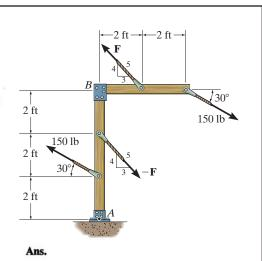
b) By resolving the 150 - Ib and 200 - Ib couples into their x and y components, Fig. a, and summing the moments of these force components algebraically about point A,
