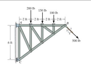
**Equivalent Resultant Force:** The 500-1b force is resolved into its x and y components, Fig. a. Summing these force components algebraically along the x and y axes,
