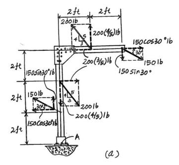
\*4–76. Determine the required magnitude of force  $\mathbf{F}$  if the resultant couple moment on the frame is 200 lb  $\cdot$  ft, clockwise.
