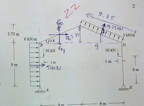
The free along AB: 6 KN/m x9 = 54 KN applied 4.5 m from A.
