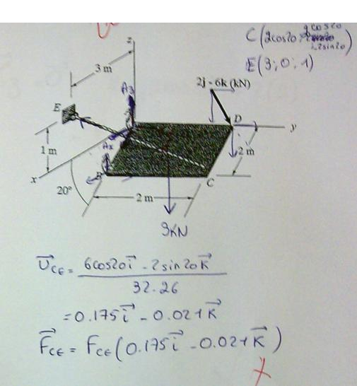
$$\begin{aligned} & \{ \vec{F}_{x} = \vec{o} \}; \quad A_{x} + B_{x} + 0.175 \text{ fce} = 0 \\ & \{ \vec{F}_{y} = \vec{o}' \}; \quad A_{y} + B_{y} + 2 = 0 \\ & \{ \vec{F}_{3} = \vec{o}' \}; \quad -3 - 6 + A_{3} + B_{3} = 0 \end{aligned}$$
