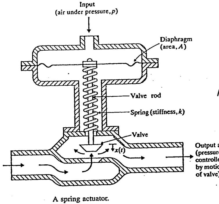
$$P_0 = \frac{F_0}{A} \Rightarrow F_0 = P_0 \times A = \frac{10 \text{ lb}}{\text{in}^2} \times 100 \text{ in}^2 = 1000 \text{ lb.}$$
