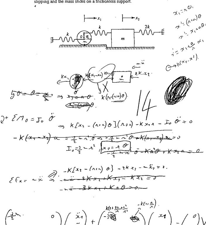
$$\det \begin{pmatrix} m\omega^2 - 3K & Ka \\ Ka. & \frac{1}{2}m^2r^2.\omega^2 + Ka^2 \end{pmatrix} = 0$$
