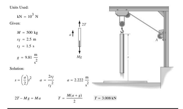
The crate of mass *M* is suspended from the cable of a crane. Determine the force in the cable at time *t* if the crate is moving upward with (a) a constant velocity  $v_1$  and (b) a speed of  $v = bt^2 + c$ .
