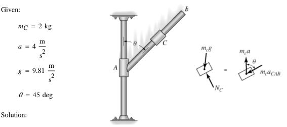
The collar accelerates along the rod and the rod accelerates upward.
