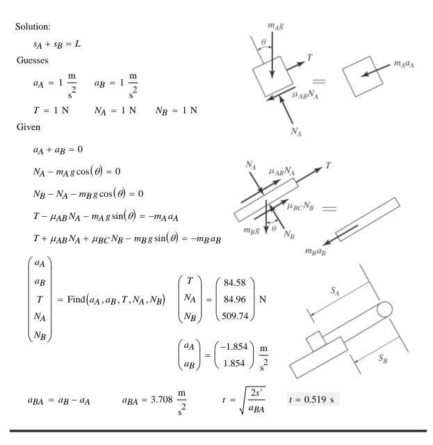
Determine the acceleration of block *A* when the system is released from rest. The coefficient of kinetic friction and the weight of each block are indicated. Neglect the mass of the pulleys and cord.
