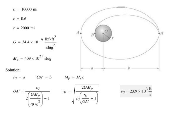
The rocket is traveling in free flight along an elliptical trajectory A'A. If the rocket is to land on the surface of the planet, determine the required free-flight speed it must have at A' so that the landing occurs at B. How long does it take for the rocket to land, in going from A'to B? The planet has no atmosphere, and its mass is 0.6 times that of the earth's.
