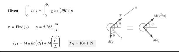
A ball having a mass M and negligible size moves within a smooth vertical circular slot. If it is released from rest at  $\theta_I$ , determine the force of the slot on the ball when the ball arrives at points A and B.
