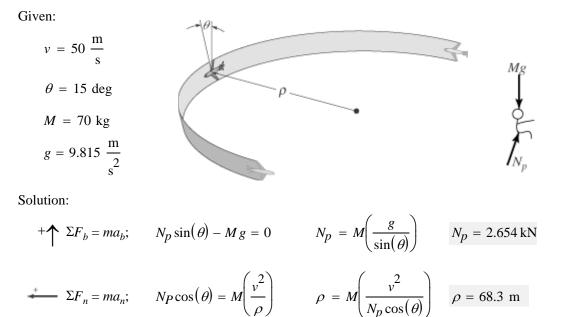
The man has weight *W* and lies against the cushion for which the coefficient of static friction is  $\mu_s$ . Determine the resultant normal and frictional forces the cushion exerts on him if, due to rotation about the *z* axis, he has constant speed *v*. Neglect the size of the man.
